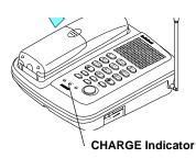
Recharge the battery pack when the handset beeps and the TALK/BATT LOW indicator flashes during a call.
